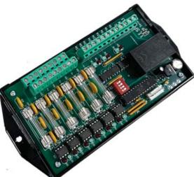
The SPR-36B operates over the standard SSI wide voltage range. The SPR-36B has a built-in low voltage transformer-isolated power supply gener
