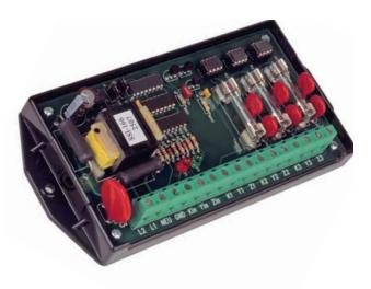
"pulled up." "Kin" is the common return. The SPR-3 may be used with meters having mechanical output contacts (relays), or high or low voltage semiconductor outputs.
