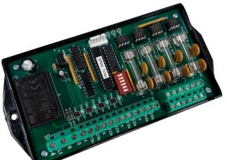
The sense voltage is sent to each meter's Y and Z terminals from the SPR-44B's "Yin" and "Zin" input terminals, returning to the "Kin" terminal, the common return for all meters. Since all meters supplying pulses to the SPR-44B have a common reference, a number of flexible input configurations can be wired. For example, two inputs can be wired in parallel giving a "splitting" configuration where one input and two outputs is desired.
