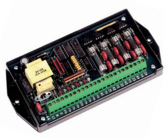
+13VDC sense voltage. The sense voltage is sent to each meter's Y and Z terminals from the SPR-44's "Yin" and "Zin" input terminals, returning to the "Kin" terminal, the common return for all meters. Since all meters supplying pulses to the SPR-44 have a common reference, a number of flexible input configurations can be wired. For example, two inputs can be wired in parallel giving a "splitting" configuration where one input and two outputs is desired.
