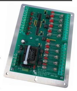
The SPR-510 relay's Form A inputs feature input fi Itering circuitry to prevent noise from false triggering the outputs. Pulses less than 18 mS are considered to be noise and will not be detected as a valid pulse. Once an input pulse, greater in length than 18 mS, is detected the corresponding outputs will be changed to match the state of the input.
