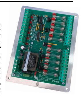
The SPR-610 relay's Form A inputs feature input fi Itering circuitry to prevent noise
