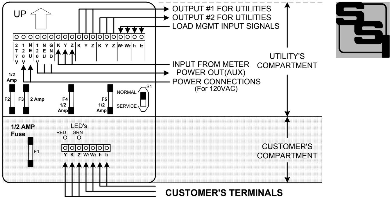
**MOUNTING POSITION** - Because the LMR-1 contains mercury-wetted relays, it must be mounted in a vertical position to operate correctly.
