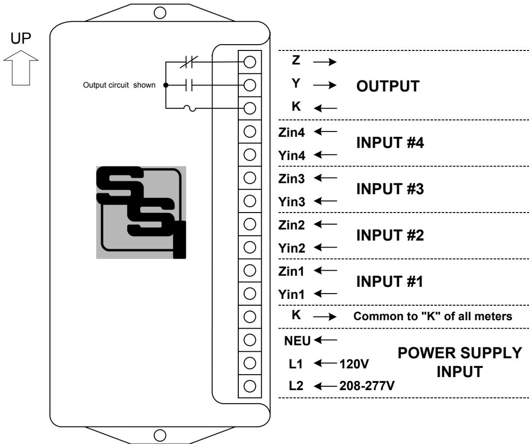
**MOUNTING POSITION** - Because the MPT-4B contains a mercury-wetted relay, it must be mounted in a vertical position to operate correctly.
