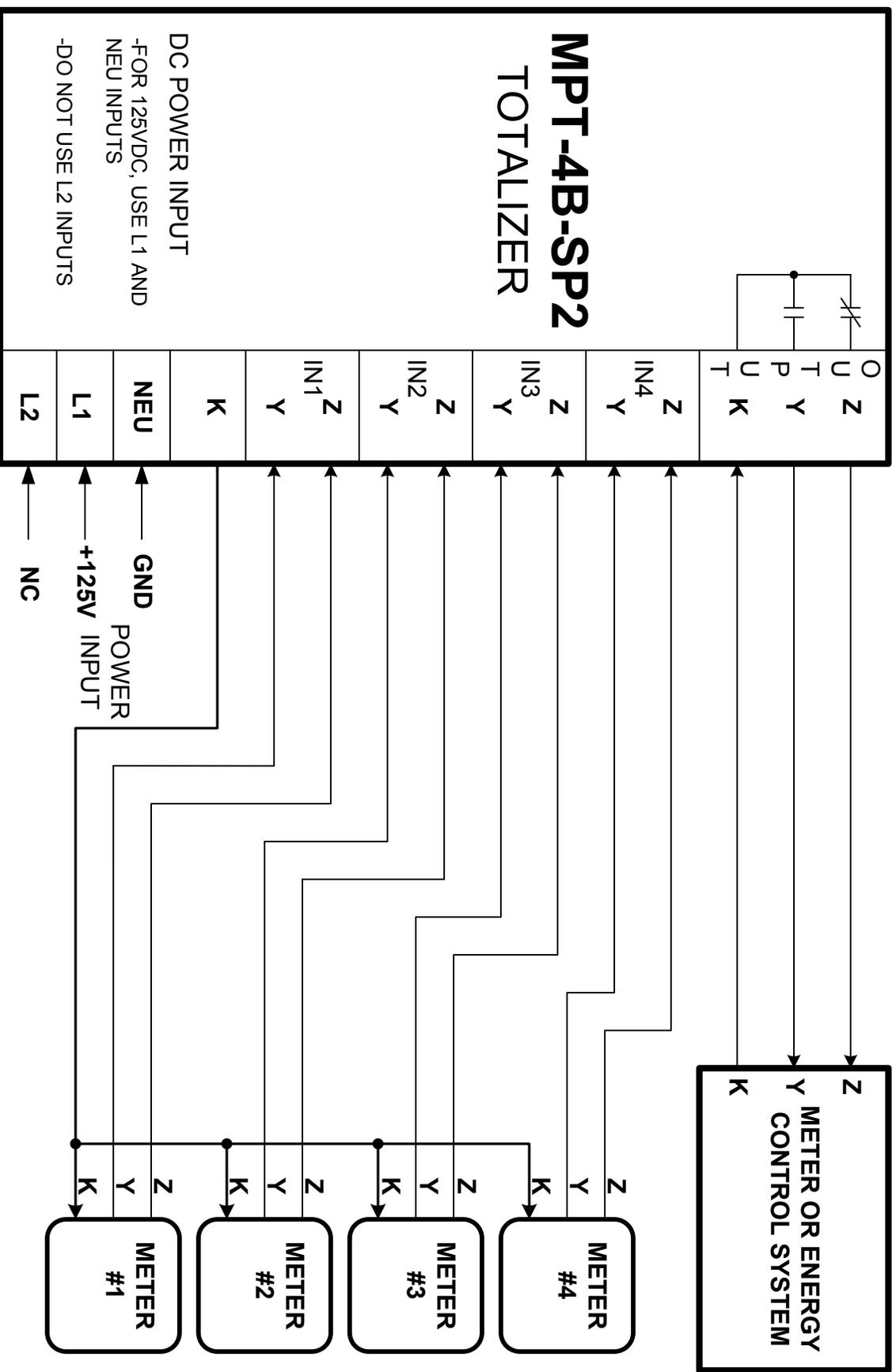
NOTE: A Sense Voltage of +13VDC is applied to the meters via the "Y" or "Z" leads from the MPT-4B-SP2. The "K" lead is the common return.
