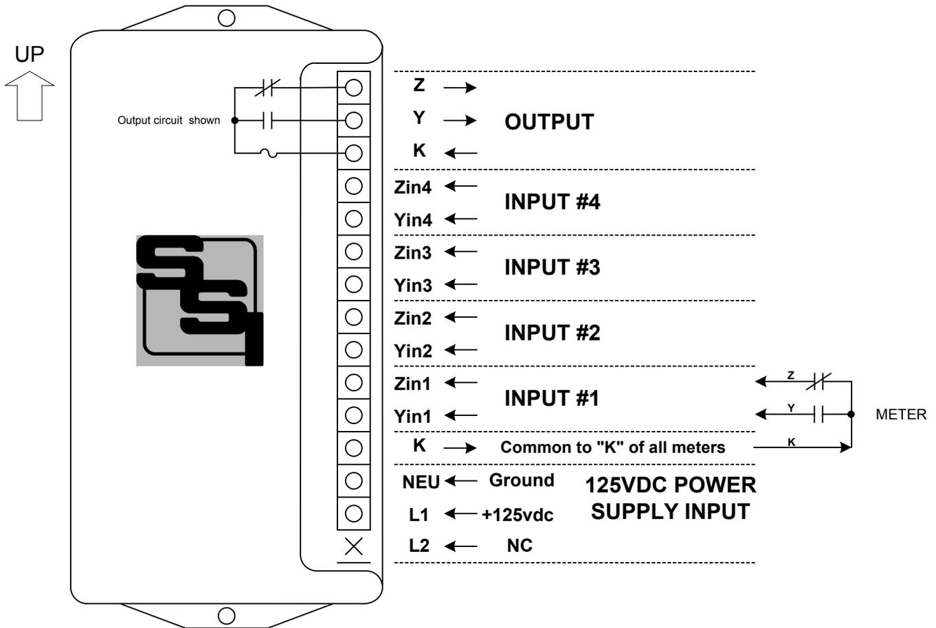
**MOUNTING POSITION** - Because the MPT-4B contains a mercury-wetted relay, it must be mounted in a vertical position to operate correctly.
