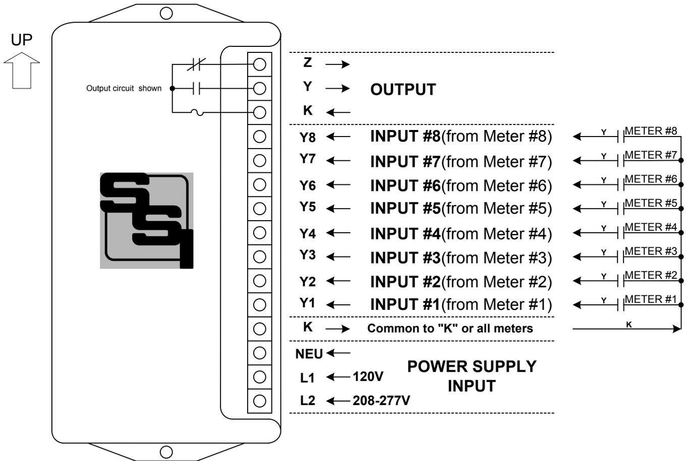
**MOUNTING POSITION** - Because the MPT-8B contains a mercury-wetted relay, it must be mounted in a vertical position to operate correctly.
