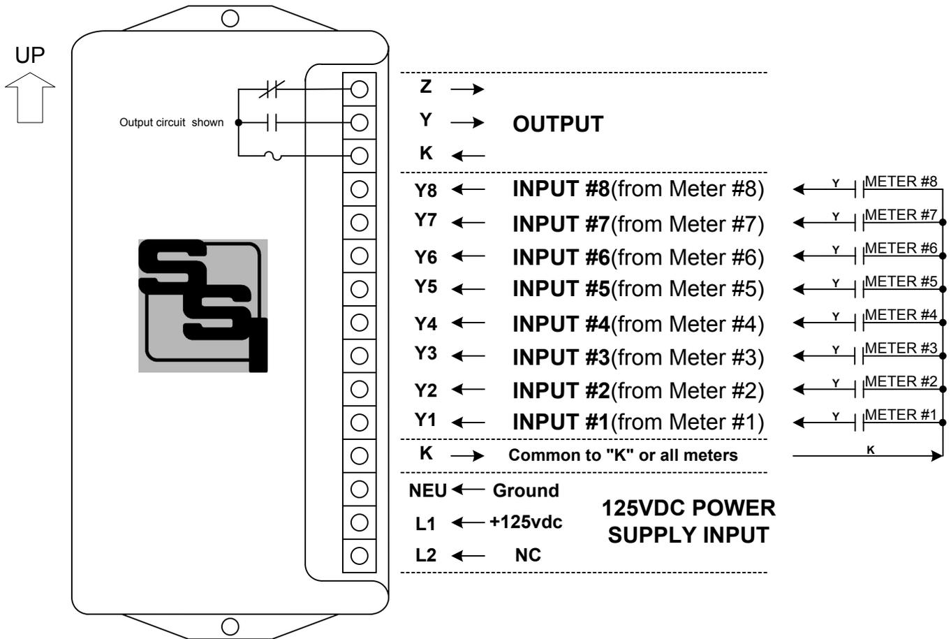
**MOUNTING POSITION** - Because the MPT-8B-SP2 contains a mercury-wetted relay, it must be mounted in a vertical position to operate correctly.
