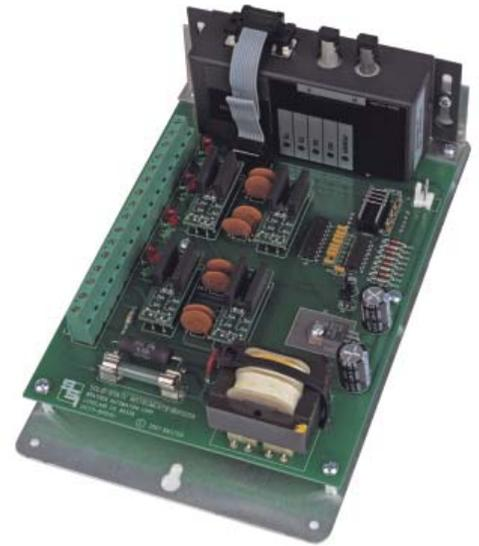
Bright red and green LEDs are included on each output of the OPR-4 to monitor each output's status. The dry contact outputs feature 1/4 amp solid-state relays for a no-bounce contact with internal MOV transient suppression circuitry to eliminate contact noise. Rapid pulse rates in excess of 20 pulses per second are possible.
