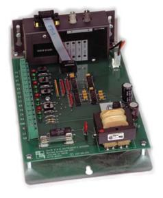
The OPT-4 transmitter is designed to receive pulses from up to four electric meters' KYZ pulse initiators. Pulses are
