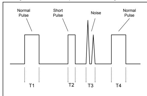
by measuring the time an input voltage is present. If the input voltage is present for less than 20 to 25 milliseconds, it is assumed to be noise. An input of longer duration is classified as a valid input and an output will occur. In the illustration to the left, the normal pulses with time durations of T1 and T4 will cause an output. The short pulse of time duration
