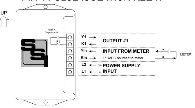
**MOUNTING POSITION -** Because the PIR-1 contains a mercury-wetted relay, it must be mounted in a vertical position to operate correctly.
