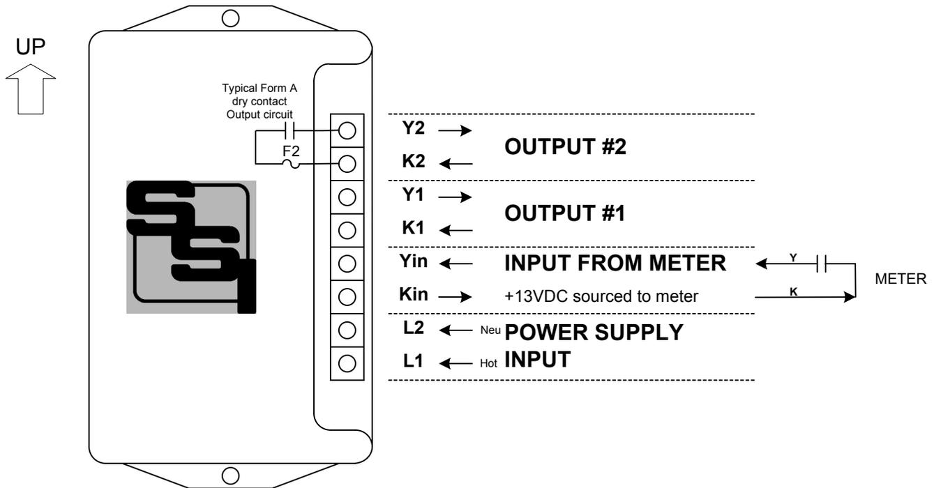
**MOUNTING POSITION** - Because the PIR-2 contains mercury-wetted relays, it must be mounted in a vertical position to operate correctly.
