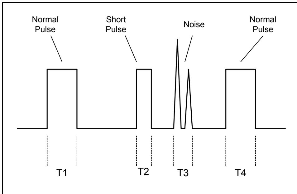
measuring the time an input voltage is present. If the input voltage is present for less than 20 to 25 milliseconds, it is assumed to be noise. An input of longer duration is classified as a valid input and an output will occur. In the illustration to the left, the normal pulses with time durations of T1 and T4 will cause an output. The short pulse of time duration
