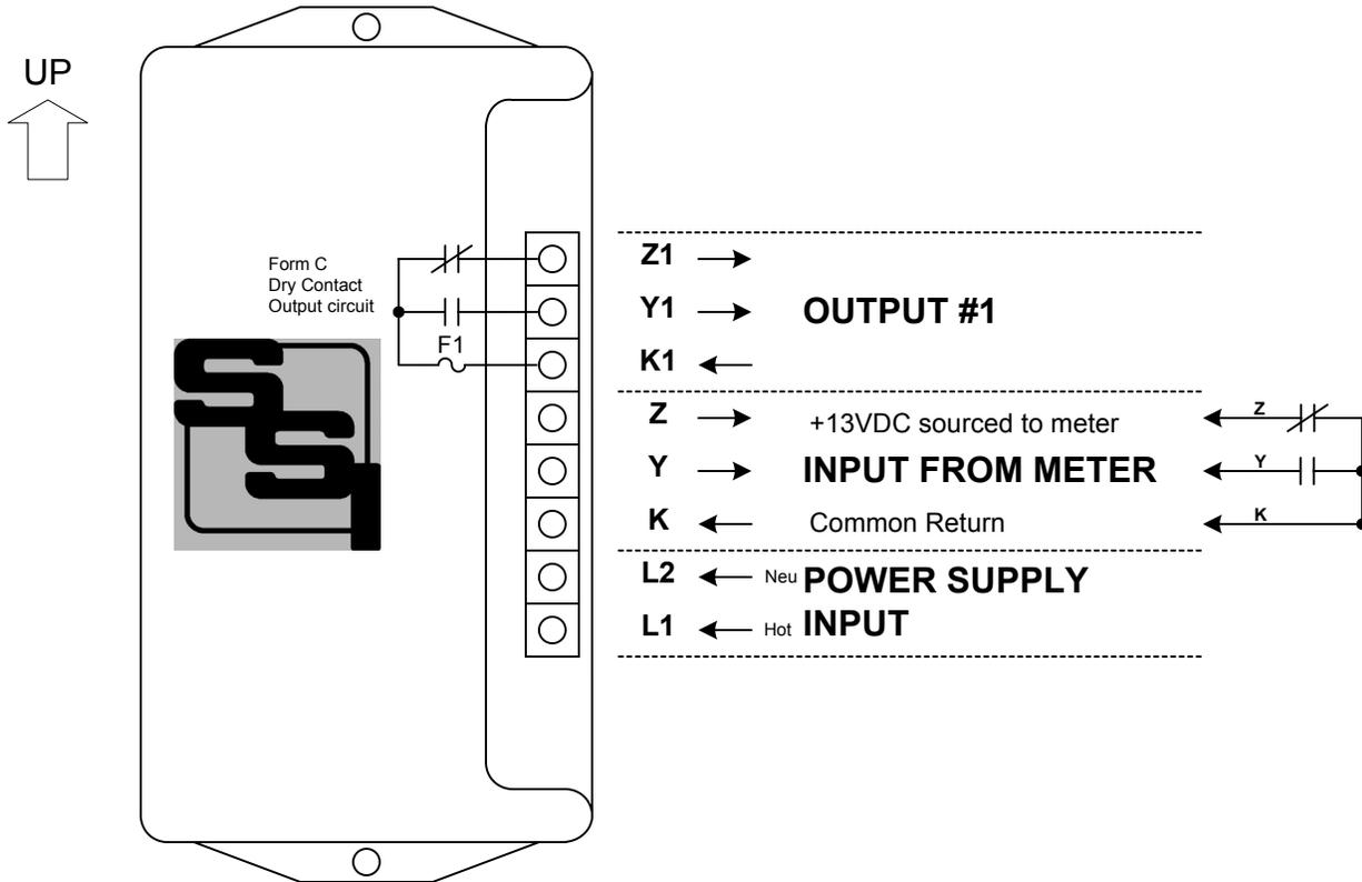
**MOUNTING POSITION** - Because the RPR-1P contains a mercury-wetted relay, it must be mounted in a vertical position to operate correctly.
