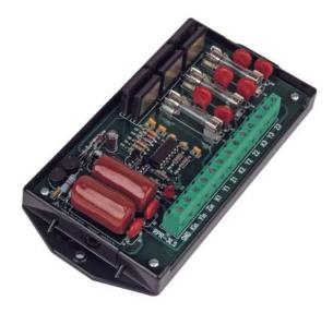
The RPR-3LS relay is designed to filter noise and transients from its input to prevent false pulses at its output. Bright red and green LED lamps indicate the system's status at all times thus allowing a rapid visual check of the system's performance without requiring any additional test equipment.
