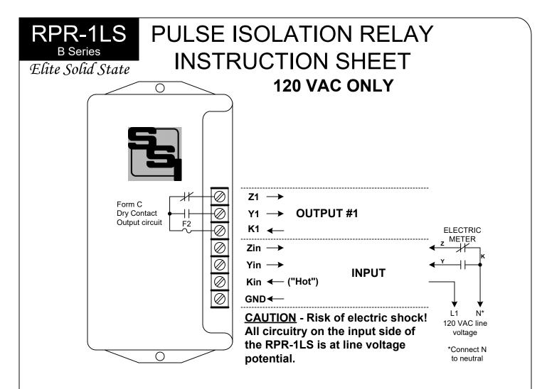
**MOUNTING POSITION** - The RPR-1LS can be mounted in any position.
